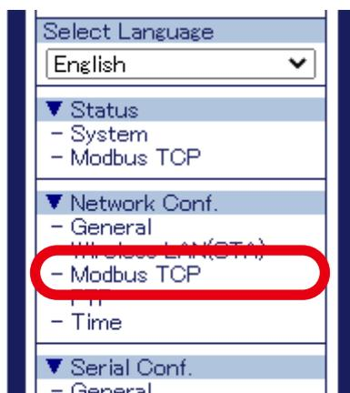
3. The **Modbus TCP Configuration** page is displayed. Configure each setting.
