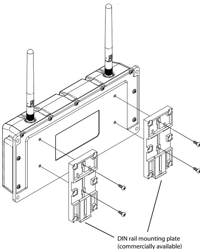
Fixing DIN rail mounting plate to DIN rail
