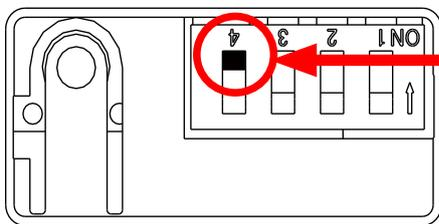
Make sure that the DIP Switch 4 is ON.
