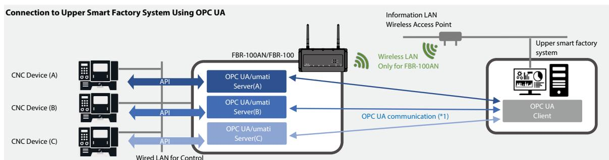
(\* 1) When reading information of multiple CNC devices from the OPC UA client, specify the number of communication port assigned to each OPC UA server.
